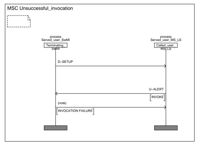
NOTE: The figure corresponds to the case where the basic call procedure continues after SS-CW invocation has failed. The case where the call is cleared because of that invocation failure is also possible (see subclause 5.4.2.2): the INVOCATION FAILURE PDU shall then be sent in the D-RELEASE PDU.
