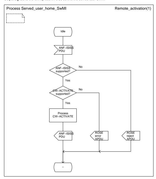
NOTE: Every ANF-ISISS PDU or ROSE APDU is conveyed by a PSS1 FACILITY message. The latter has not been shown in the corresponding signal symbols by lack of space.
