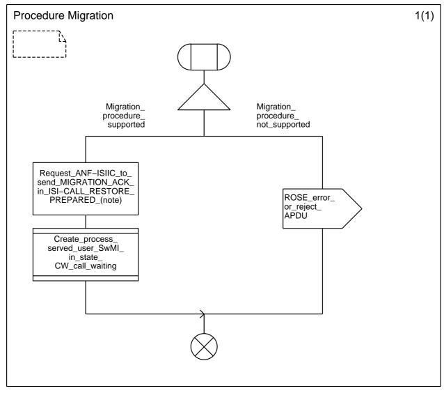
NOTE: ANF-ISIIC may delay the sending of the ANF-ISIIC-CALL RESTORE PREPARED PDU by a few seconds. If the served user decides to accept the waiting call during that time (in sending the U-CONNECT PDU), ANF-ISIIC may skip the sending of the ANF-ISIIC-CALL RESTORE PREPARED PDU in sending directly the ANF-CONNECT PDU. In such a case, the MIGRATION ACK PDU will not be sent.
